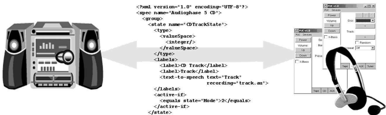
Figure 1. A diagrammatic overview of the personal universal controller system, showing an appliance, a snippet from our specification language, and two graphical interfaces generated from the specification.
