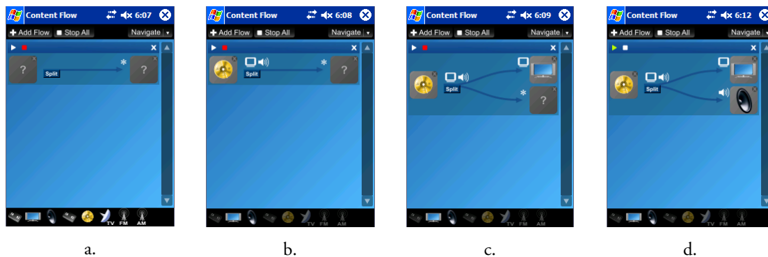
Figure 9.3. An example of using the Flow-Based Interface to configure a DVD player to play video through a television with the audio routed through the stereo's speakers.
