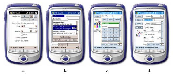
Figure 1.2. Interfaces generated by the PUC on the PocketPC for several different appliances: a) Windows Media Player 9, b) the navigation system from a 2003 GMC Yukon Denali, c) the Canon PIXMA MP780 all-in-one printer, and d) the HP 2610 all-in-one printer.
